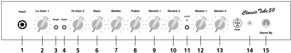
**1 Input:** Input  $\frac{1}{4}$ " unbalanced input. Plug your guitar cord in here.
