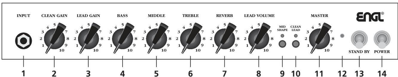
**1 Input:** ¼" unbalanced input jack. Plug your guitar in here using a shielded cord.
