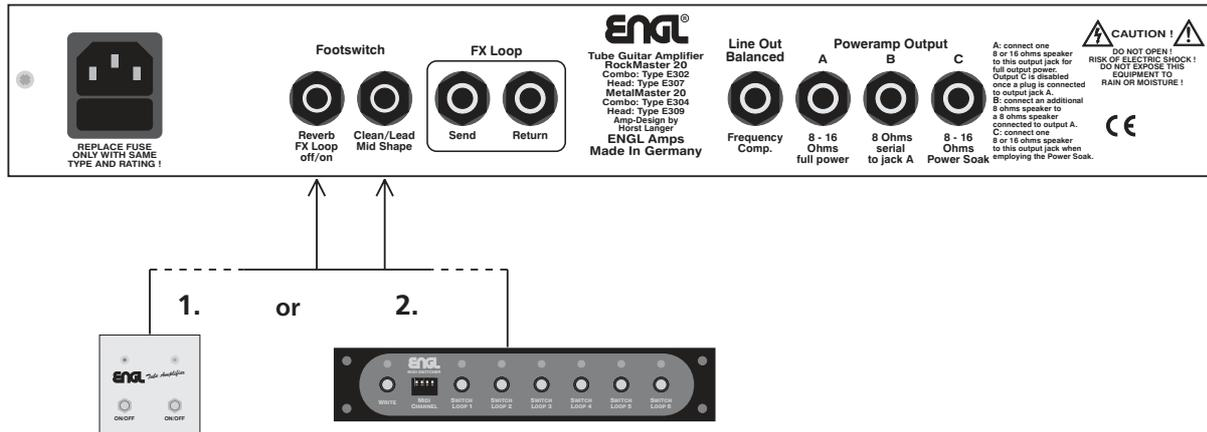
1. Use a dual footswitch such as the ENGL Z-4, connecting it to the amp via a stereo cord equipped with 1/4" jack plugs. You can switch channels and *Mid Shape* via the dual footswitch connected to port 18, *Reverb Off/On* and *FX Loop off/on* via the dual footswitch connected to port 17.
